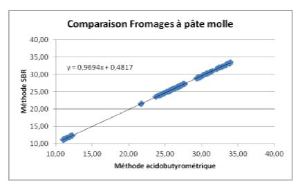
The regression equation  $Y = 0.9694 \ X + 0.4817 \ was obtained between the methods (see graph above) with a mean difference of +0.30 g of fat/100 g for this type of cheese (Extraction: 25.23 g/100 g – Acido-butyrometry: 25.53 g/100 g)$
