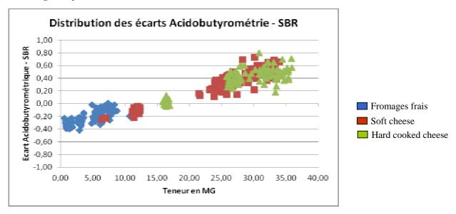
When all the various cheese types were integrated in the regression, an equation between the methods Y = 0.9741 X + 0.3451 was obtained with a mean deviation of +0.18 g / 100 g. Deviations from -0.40 g / 100 g to +0.80 g / 100 g of cheese were observed which are closely linked to the fat concentration of the product.
