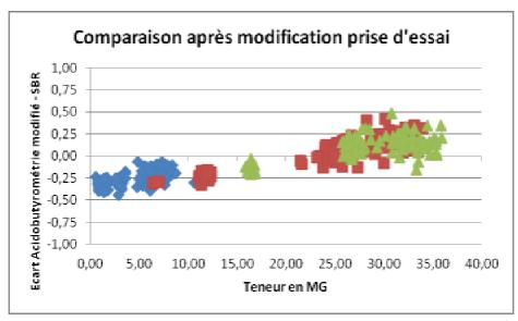
Although after correction of the results an improvement and a decrease in the deviations between the methods was observed (about -0.40 to +0.40 g /100 g), this type of modification to the operating procedure does not enable the difference observed to be resolved over the entire fat content range within the field of application of the method tested.
