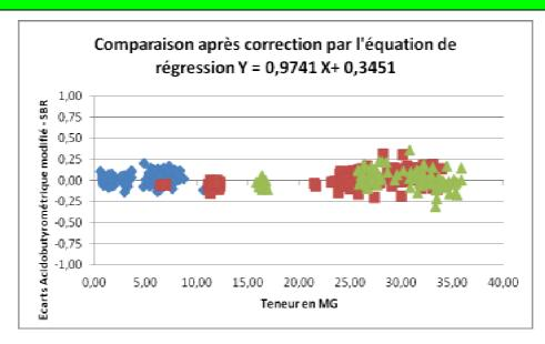
Applying a correction equation ensures the traceability between the methods in all fields of application of the method. No systematic difference specific to cheese types tested was observed. The accuracy estimate (calculated by 2.Sy,x: residual standard deviation of regression) of the acido-butyrometric method in relation to the SBR reference method is  $\pm$  0.18 g / 100 g.
