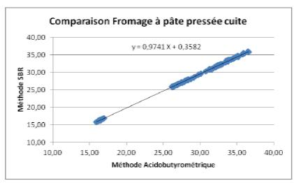
The regression equation  $Y = 0.9741 \ X + 0.3582$  was obtained between the methods (see graph above) with a mean difference of +0.39 g of fat/100 g for this type of cheese (Extraction: 28.56 g/100 g – Acido-butyrometry: 28.95 g/100 g)
